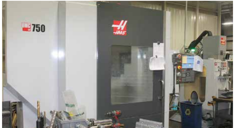
Above: A Haas UMC-750 5-Axis machining center at Creative Blow Mold. Find video at the company's website: http://creativeblowmold.com/5-axis-machining-advanced-technology/
