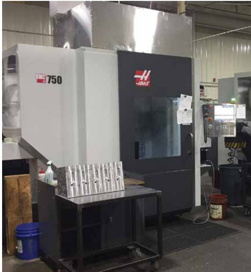
Above: One of two Haas UMC 750 5-axis machining centers at Creative.
